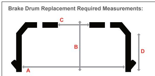
For an accurate replacement of the brake drum, it's essential to take precise measurements:
